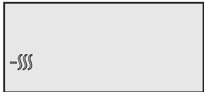
Drying level damp
